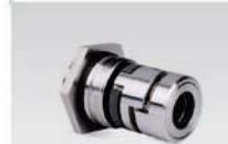
Balanced & container-type shaft seal with all the parts assembled together, no axial rotating to prevent the shaft and rubber parts from wearing, with the characteristics of rapid changing, easy installation and safe operation. Dynamic sealing is made of cemented carbide materials and the static sealing is fluorine rubber material which make the mechanical seal to be high temperature resistance, long service life, easy changing and other significant characteristics.
