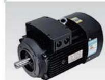
High-efficiency standard motor, Japan NSK bearings and cold-rolled 50ww800 silicon steel sheet made the pump high efficiency, low noise and maintenance-free. Totally enclosed shaft seal, IP55 protection grade, F class insulation grade, the special "double-lock" drive end bearing made the pump withstand higher inlet pressure.
