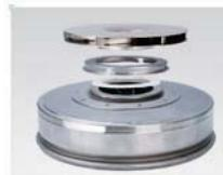
The built-in floating sealing ring of the pump cavity body could minimize the internal leakage produced by the differential pressure and prevent the energy consumption when liquid leaking back to the pump cavity body.
